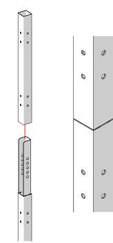
POST, EXTENSION POST, AND SPLICE BRACKET ARE SECURED WITH HARDWARE THAT IS INCLUDED WITH PANELS
