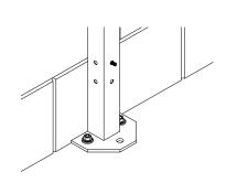
STANDARD INSTALLATION - 2 ANCHORS PER BASEPLATE REQUIRED
